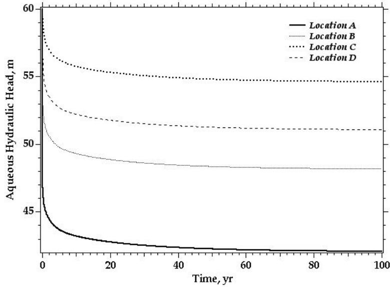
Figure 5. Hydraulic head in response to pumping
