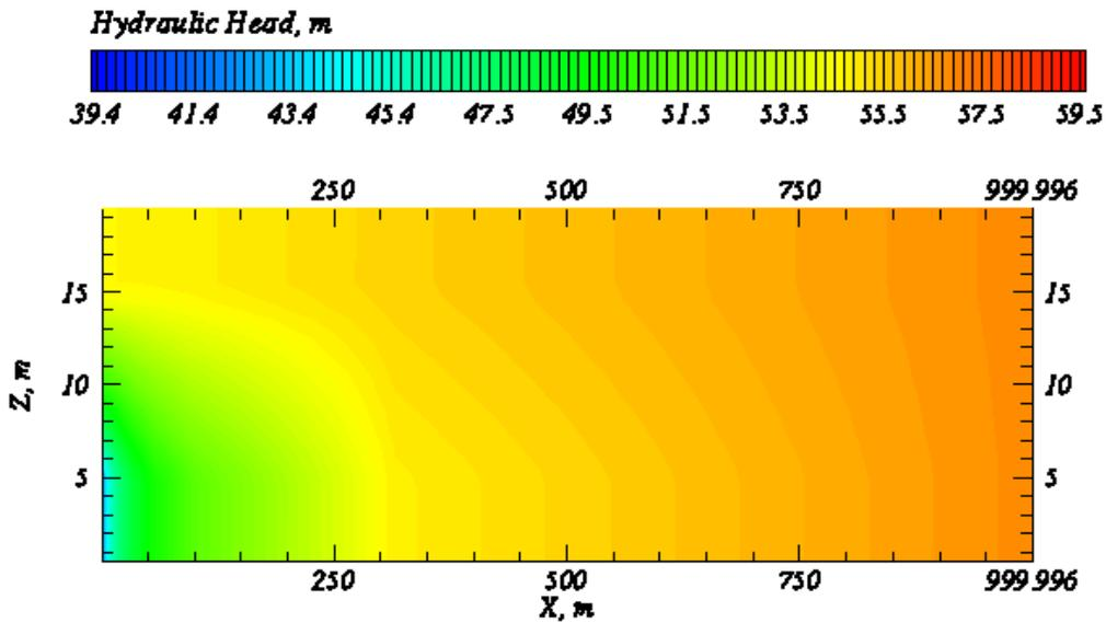
**Figure 7.** Contours of hydraulic head in response to pumping (10:1 anisotropy ratio)
